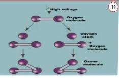
Ozone is generated electronically using high voltage corona effect. A colorless tri-atomic oxygen gas.
